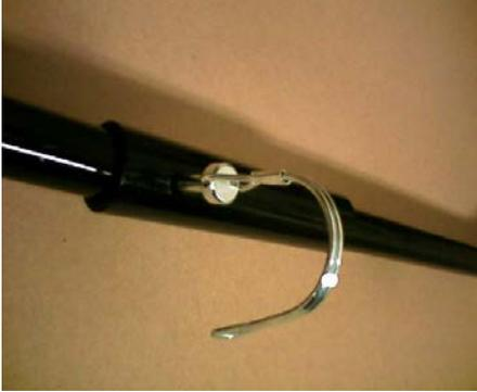
**Step 1:** Slide the stand's smaller top horizontal tube into the opposite larger top horizontal pipe, align the holes, insert lynch pin through the holes and latch the locking loop over the exposed end of the lynch pin.
